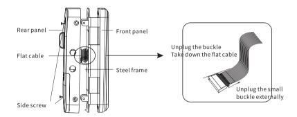
Notes: Prop the rear panel with your hands when unscrewing the screw and then take away the rear panel after the disassembly of the flat cable.
