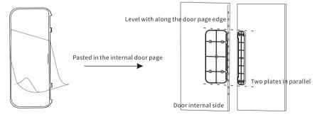
You can begin the installation of the lock body after the flitch plate is aligned. First unscrew the screws on the side of the lock body and then take off the rear panel.
