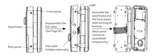
Remarks: Please pay attention to the flat cable connection when unscrewing the screws on the rear panel. Please disassemble the flat cable first, then connect it with the rear panel and conduct subsequent operation.
