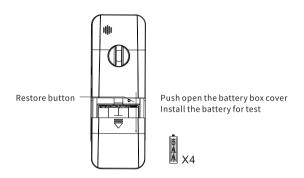
Test: Gently touch the screen buttons after battery installation(press any key for wake up) and see whether there is any reflection. Please carry out the following procedures if there is no reflection.
