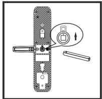
(4) Adjust the handle direction according (5) Insert square bar into front handle, the dot should point to upward side.
