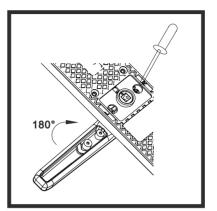
to the door open direction, if change open direction need to loosen the screw to adjust handle 180 degrees
