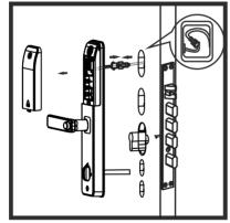
⑦Install back plate, connect the square bar, the knob insert to the mortise hole and connect cables.
