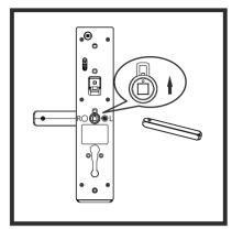
④Adjust the handle direction according ⑤ Insert square bar into front handle, the dot should point to upward side.
