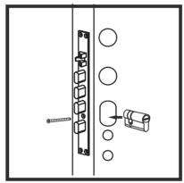
③Install cylinder and fix the cylinder with screw.
