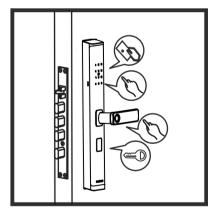
(1) Test the installation by inner handle, knob, mechanical key, and password, password and fingerprint.
