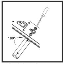
to the door open direction, if change open direction need to loosen the screw to adjust handle 180 degrees
