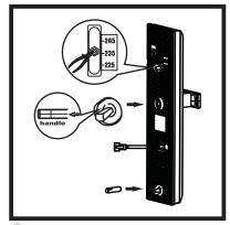
Adjust upper screw sleeve according to actual door hole position. Insert square bar into handle hole, make sure arrow points to handle direction.
