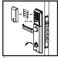
Install the battery box and batteries, test the deadbolt.
