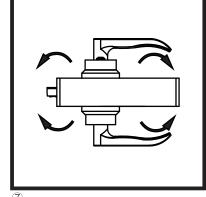
Adjust face plate position to make sure it is straightly and correctly installed.
