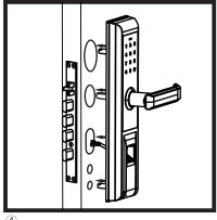
Install front faceplate, making sure different parts go into correct holes.
