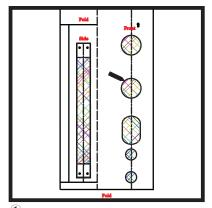
Place the template on the door. According to the template,mark the holes on the door with a pencil.
