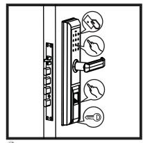
Test the installation by inner handle, knob, mechanical key, fingerprint, password and reading card.
