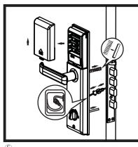
Install back faceplate, don't forget to put the spring inside the handle and connect cables.
