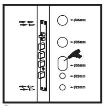
Take out the mortise before drilling the holes. Drill the door hole with a driller of 20mm and 35mm for mortise. Fix the mortise with screws.
