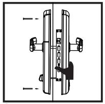
Use one hand to press front faceplate against the door, fix back faceplate with 2 screws.
