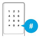
e Input "#" again to confirm and the "double unlocking mode" is disabled.
