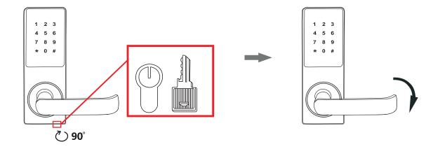
The mechanical key cannot unlock the lock directly.
